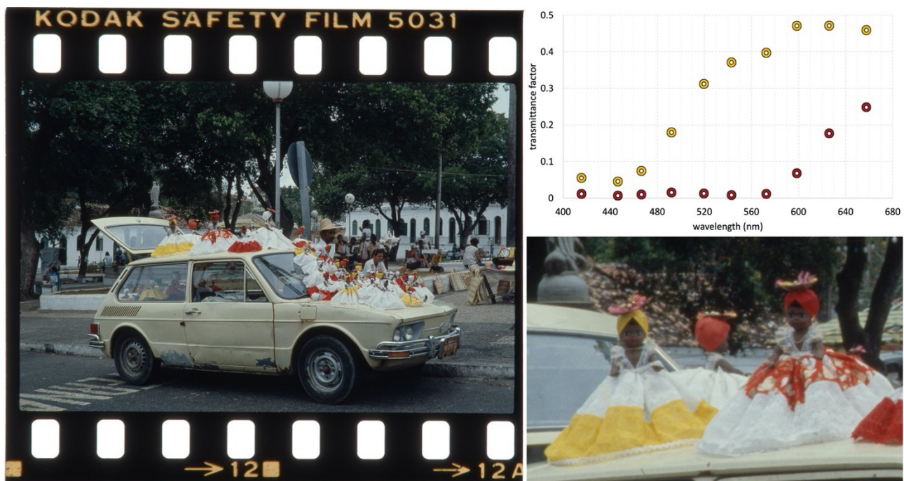
Fig. 3 - An edge-to-edge multispectral capture of a slide with the LED-based system (left). Bottom-right: Image detail of the car roof. Top-right: Transmittance values corresponding to the yellow skirt of doll on the left and to the red turban of the doll on the right. Courtesy of the Art Institute of Chicago.
