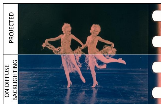
Figure 1: Different appearances of a tinted and toned film (“Tänze”, 1920 from the Deutsches Filminstitut - DIF) when projected (top) and when observed in diffuse illumination (bottom).
